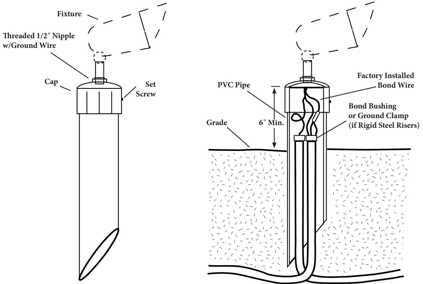
**READ AND UNDERSTAND THESE INSTRUCTIONS BEFORE INSTALLING FIXTURE.** This fixture is intended for installation in accordance with the National Electrical Code and local code specifications. To prevent electrical shock, turn off at fuse box before proceeding.
